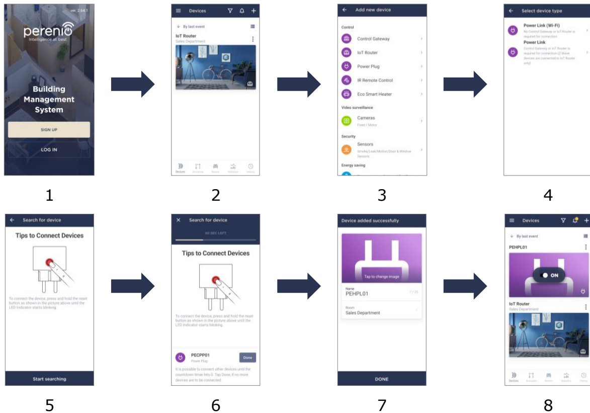
Figure 5 – Activation of Power Link (Zigbee)
